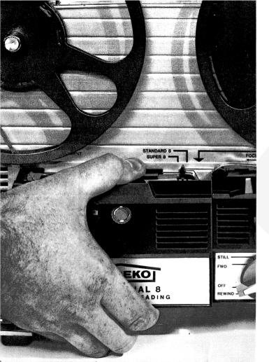
**DAMAGED FILM:** For trouble-free projection, your film must be in good condition. Cut out bad sections of film which have torn perforations, and make certain all splices are aligned and in good condition. Repair poor splices before showing movies to your audience. Film which does not feed through the projector because its perforations are torn or damaged must be removed from the projector for repair.
